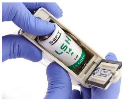
Figure 9: Insert a new battery according to the polarity. The battery removal strip underneath the battery facilitates easier removal.
