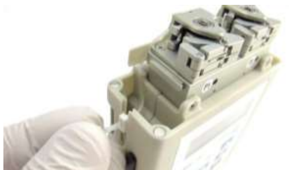
b: Tubing with strain relief is placed into the slot located on the left side of the pump.
