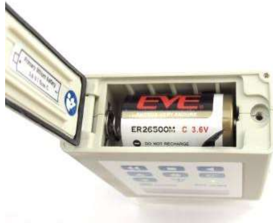
Figure 22: Inserting the new battery
