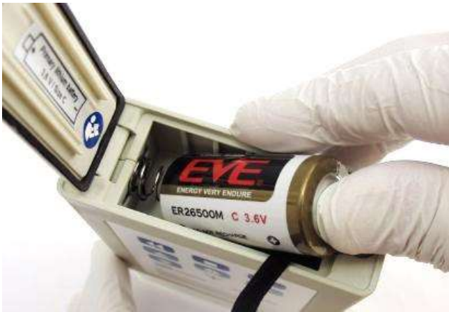
Figure 8: Insert a new battery according to the polarity. The battery removal strip underneath the battery facilitates easier removal.
