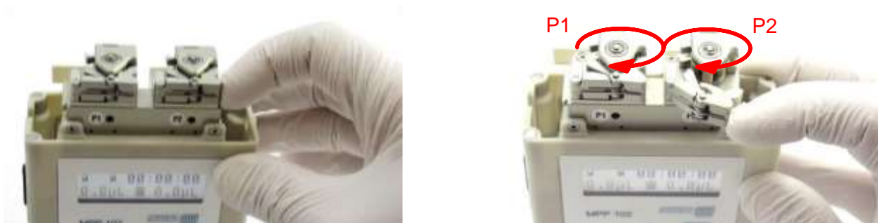
Figure 14: Opening of pump head using the snap mechanism.
