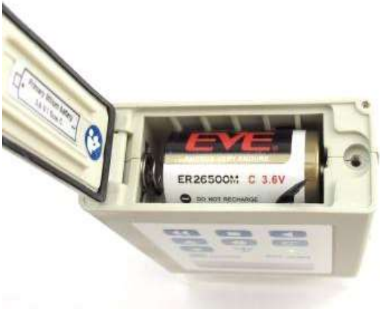
Figure 9: Insert battery with pressure against the spring, positioning battery removal strip, and then closing the battery compartment cover with a T10 Torx key by securing the battery compartment screw.
