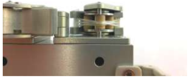
b: Tubing set inserted INCORRECTLY
