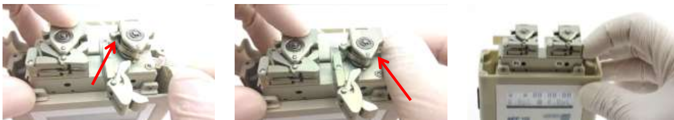
Figure 15: Inserting the tubing into the pump module
