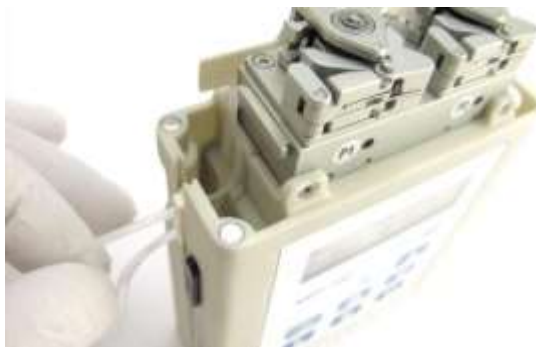
Figure 18: Tubing set placed in the slot of the pump with fixed strain relief
