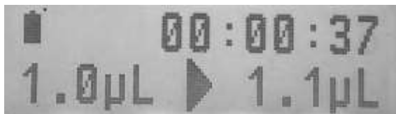
Figure 21: Home screen: Double lined display during pump / flush mode
