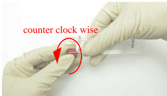
Figure 2: Remove red protection cap from the perfusate bag
