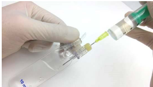
Figure 4: Filling the perfusate bag via injection port
